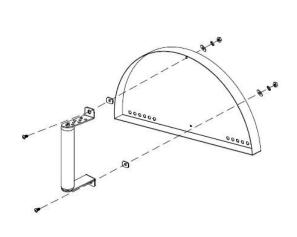
6/. Installed chimney cap with 4pcs of 5/32"\*10mm screws
