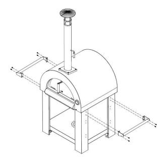
10/. Installed 3pcs of hooks 1 and 1pc of hooks with 8pcs of 1/4"\*15mm screws
