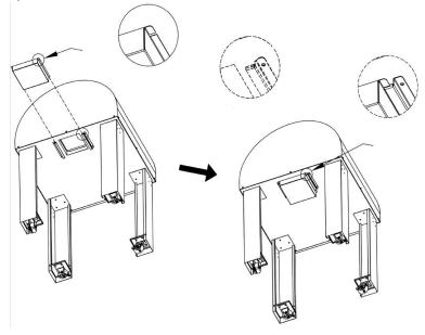
5/. Installed the door handle with each 2 pcs of 1/4"\*15mm screws + insulation mat + flat washer + spring washer + 1/4" bolts
