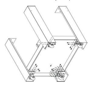
2/. Fasten legs on the oven body with 12pcs of 1/4"\*15mm screws
