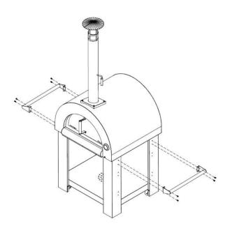
**7.** Install left and right handle with 8pcs of 1/4"\*15mm screws.
