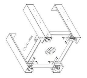
**1.** Install the bottom shelf with the 16pcs of 1/4" \*15mm screws. Make sure swivel casters w/ brakes are on the right or left side of the unit.
