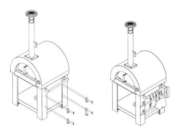
**8.** Install 3pcs of hooks 1 and 1pc of hooks with 8pcs of 1/4" \*15mm screws.
