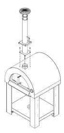
**6.** Install chimney box with 4pcs of 1/4" 30m screws.
